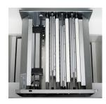
FanFold-D V5 is a high-speed single-tractor-feed braille printer at a truly affordable price. It combines an excellent dot quality, high speed, and low maintenance cost.
